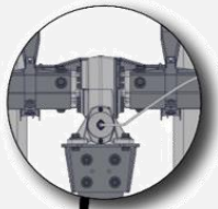
Centre HEA Pile & Drive
